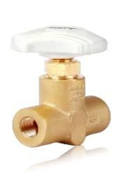
The Mack short stem cryogenic cylinder valve has been designed from the ground up, to provide a robust and dependable shut-off device for use on portable cylinders. Its clever design enables it to move from fully closed to fully open, without changing the overall height, making it perfect for application in the tight confines of a liquid cylinder.
